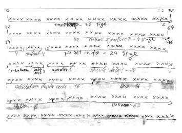
Figure 3: Mapping of the data stored on each Event log record.
